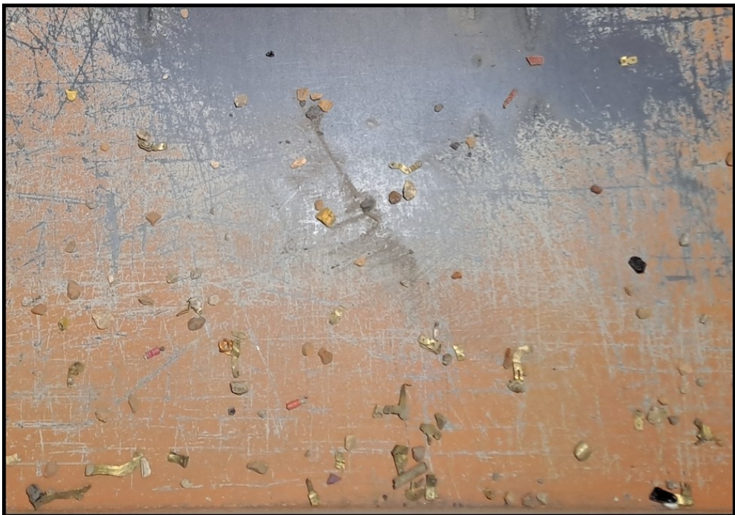
Figure 20: Cu/Brass Concentrate from optical separator at Spectra Media.
