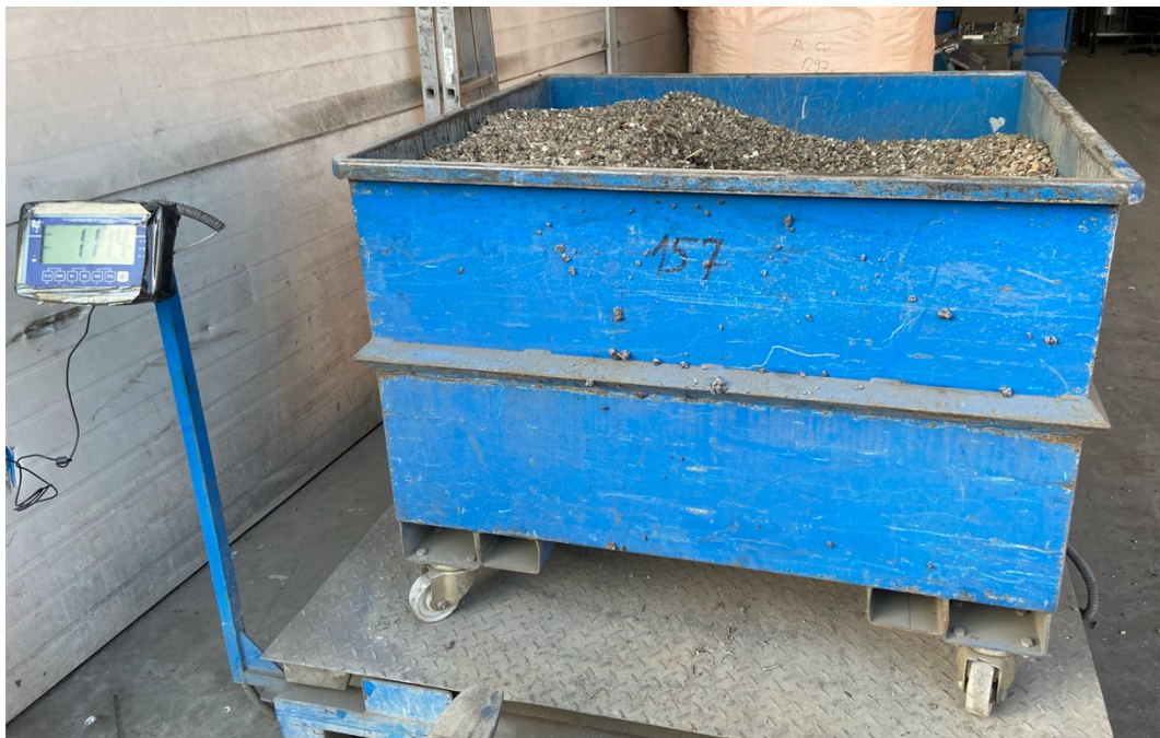
Figure 12: Feed sample for optical sorting process at spectra media.
