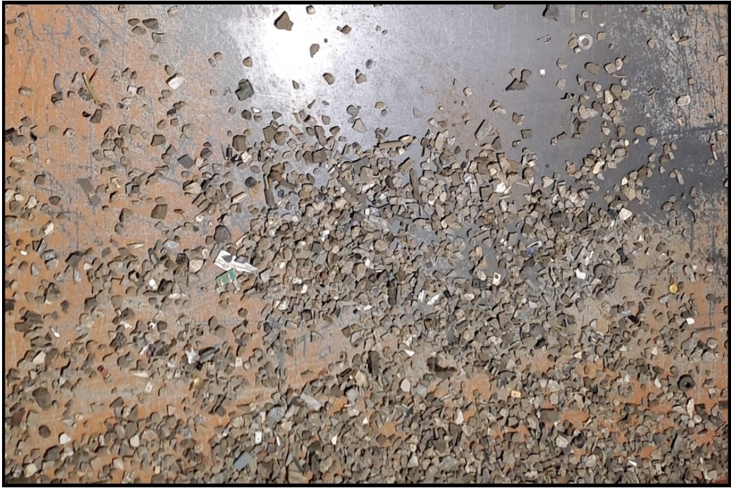
Figure 19: Aluminum concentrate from Optical separator at Spectra Media.
