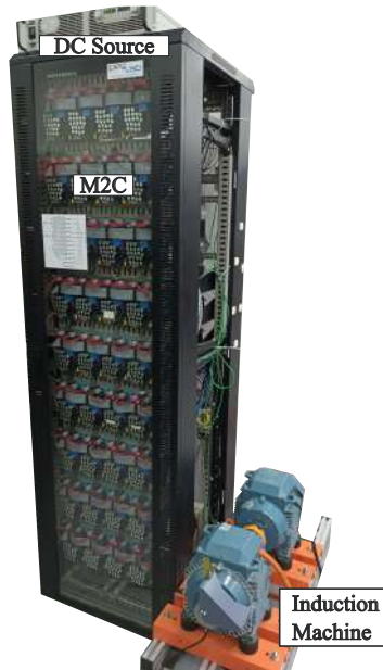
FIGURE 4.1: Experimental setup composed of the MMC (M2C) converter, DC current source, and induction machines coupled together.
