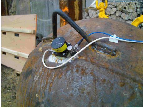
(a) Accelerometer on the iron ball
