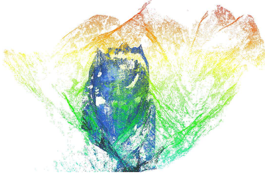
FIGURE 6.24. 3D LiDAR points before the collapse (IGN survey displayed in height color scale) and after the collapse (Helimap survey - blue points)
