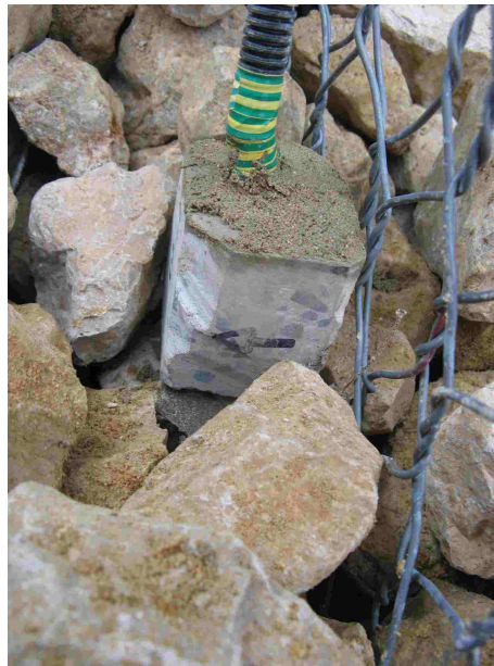
(c) Accelerometer inside a gabion
