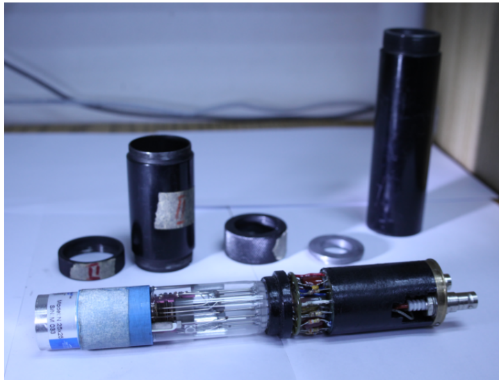
Figure 3.4: Detector housing, photomultiplier and BrillLance crystal.
