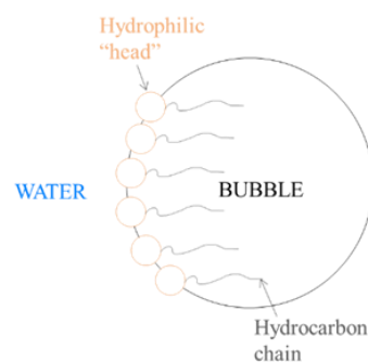
Figure 8. Structure and interfacial orientation of a frother molecule at the air-water interface. Modified from Wills & Finch (2016).
