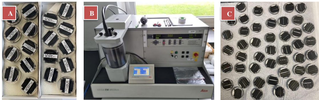
Figure 17. Epoxy samples for MLA (A); Carbon coating device (B); An image of carbon-coated epoxy samples (C).
