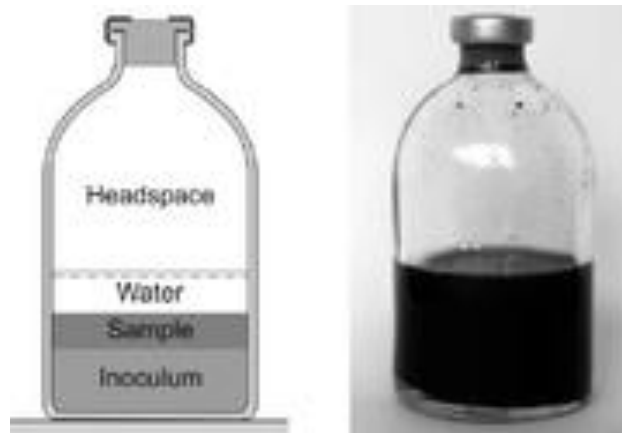
Fig. 2.3. Image of a bottle for a BMP type test along with a sketch of the parts that are requested in the bottle.
