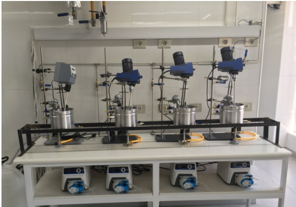
Figure 13: implementation of the proposed benchmark system in the laboratory. It can be seen the four units with their respective instrumentation.
