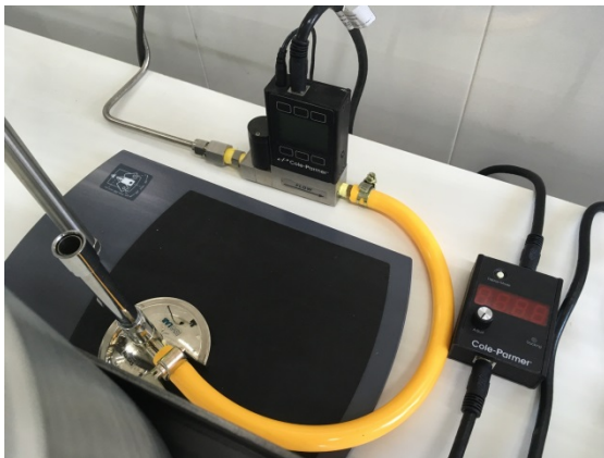
Figure 15: View of the lighter and its gas mass controller. On the side is the controller's set-point unit.
