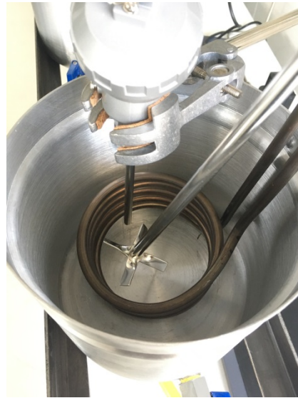
Figure 14: Top view of the unit one. It can be seen the agitator, the resistance and the thermocouple.
