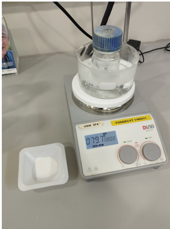
Figure 2.1: Preparation of PVA solution in ultrapure water at 80 degrees Celsius, heater plate, PVA in white plastic pot.
