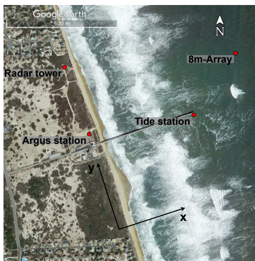
Figure 4.2: FRF site at Duck, NC, with local coordinate system and reference location of sensors (©2013 Google Earth).
