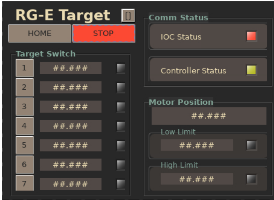
Figure 21: RG-E CS-Studio main screen. The HOME and A, B, C, etc buttons move the target strip to the corresponding location, the STOP button is an emergency, instant stop of the target system, and the Motor Screens button allows the user to open additional motor screens.
