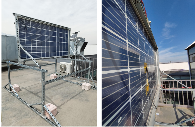
Figure 4.4: Outdoor setup (left) vertical module oriented east-west and (right) close-up of temperature sensor and pyranometers installed on the rear surface.
