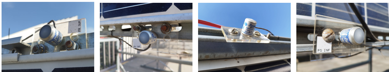
Figure 4.6: Four pyranometers for frontal and rear irradiance measurement.
