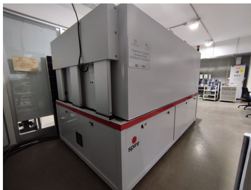
Figure 4.2: A+A+A+ sun simulator used for indoor measurements.
