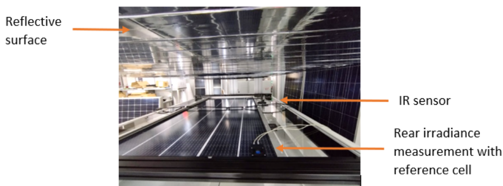
Figure 4.3: Sun simulator with elevated cabin and a reflective film in its surface.
