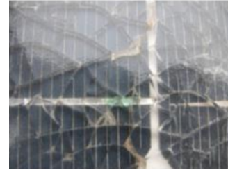
Figure 2.1: Glass breakage in a module [5]
