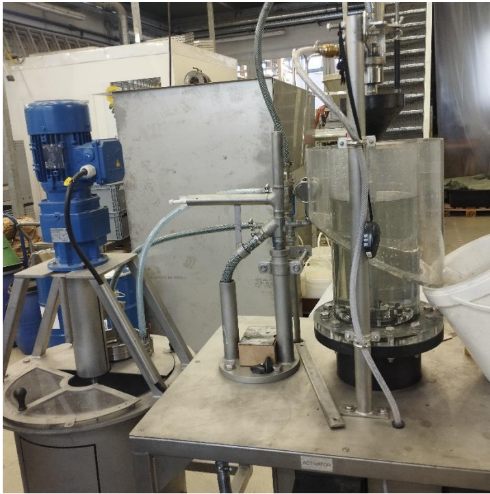
Figure 6. Allmineral pneumatic cell with separate conditioning unit.
