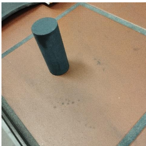
Figure 26. Sample of pellet produced from pressure agglomeration.
