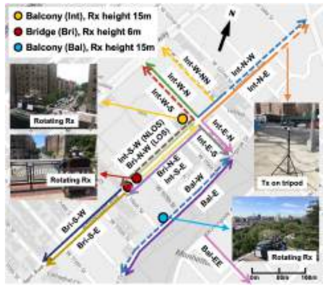
Figure 1: Locations and example street views of the three measurement sites in the COSMOS testbed deployment area. The receiver (Rx) is placed at a fixed location in each site (marked by a circle), and the transmitter (Tx) is moved along the measurement sidewalks (marked by lines). Solid and dashed lines correspond to sidewalks (or part of the sidewalks) where the Tx and Rx are in line-of-sight (LOS) and non-line-of-sight (NLOS), respectively.
