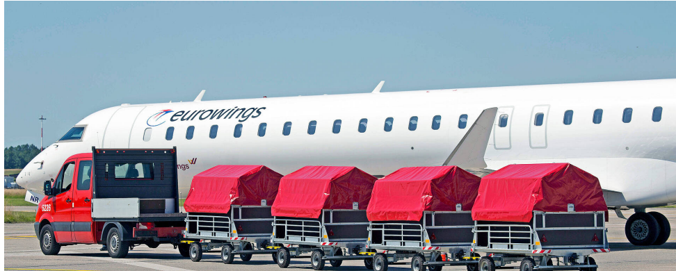
Figure 2.1: Luggage N-Trailer used in airport operations. Source: www.gse.blumenbecker.com
