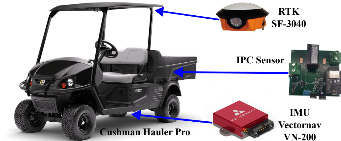
Figure 2.25: Electric vehicle used for field testing, equipped with an RTK GNSS system, an IMU, and a voltage/current sensor connected to the batteries for IPC measurement.
