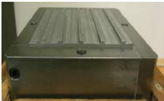
Fig. 3. Example of BCR3D bottom box with a solid steel plate with shear keys
