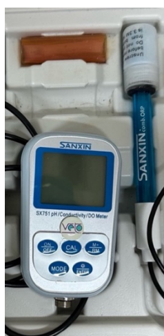
Figure 12. San-Xin SX751 meter with ORP electrode.
