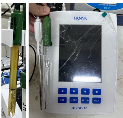
Figure 13. HI5522 multi-parameter with conductivity, temperature, and pH probes.
