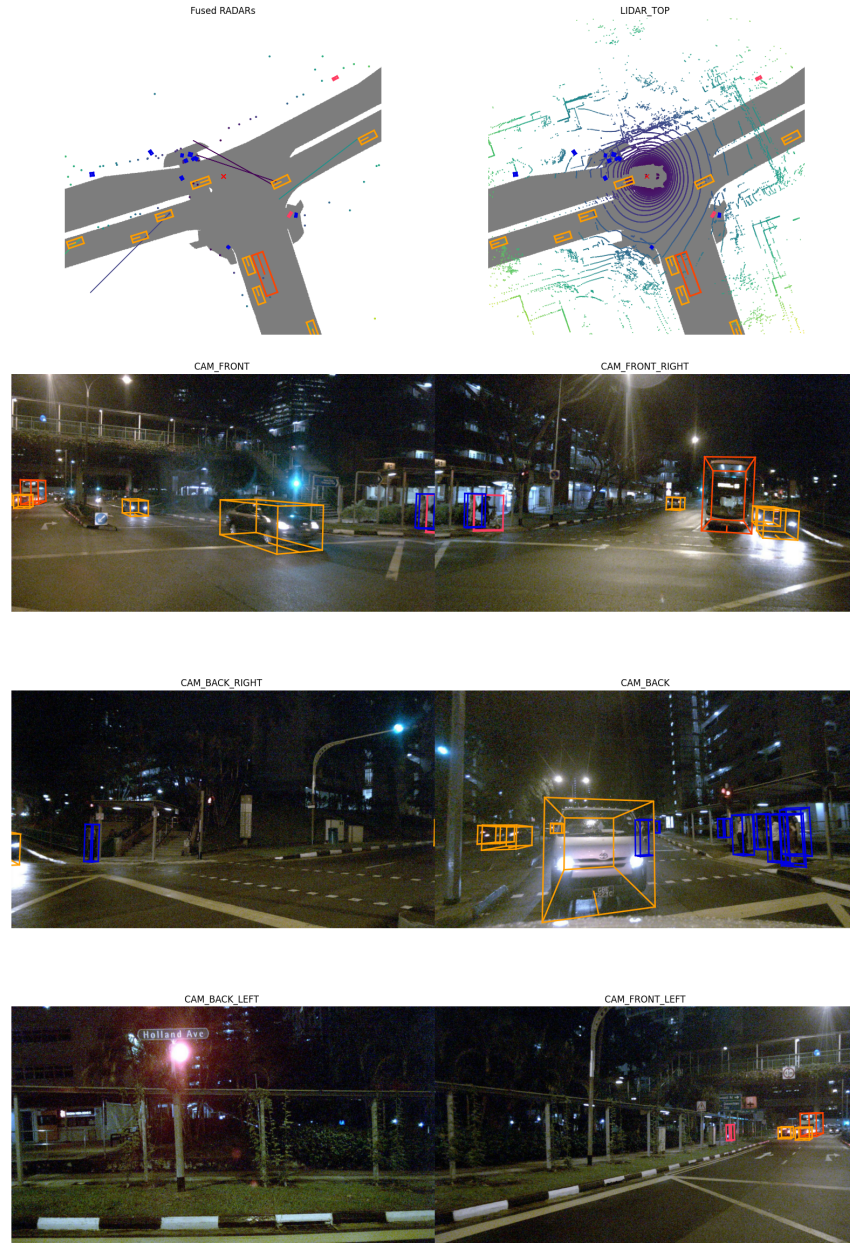
Figure 5.1: NuScenes Sensor Data (Night). Example of nighttime multi-sensor data from NuScenes, including several camera viewpoints along with RADAR and LiDAR top-down overlays. Bounding boxes (orange/blue) indicate detected objects in low-light conditions.
