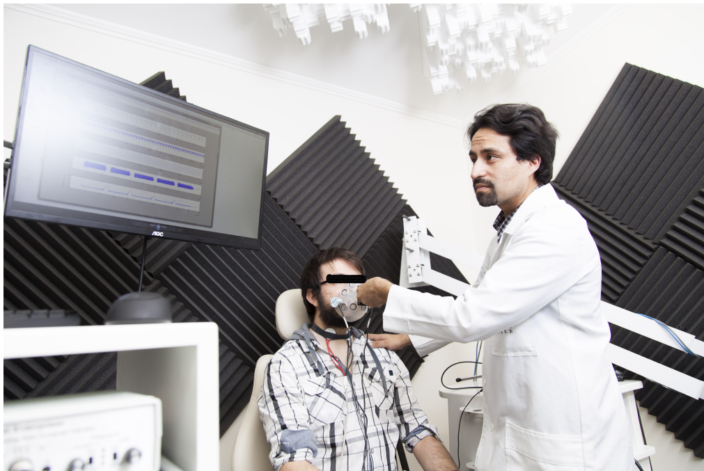
Figure 2.4: Extraction of aerodynamic measurements with a Rothenberg mask. Voice Production Laboratory (VPLAB), Universidad Técnica Federico Santa María, Valparaíso, Chile
