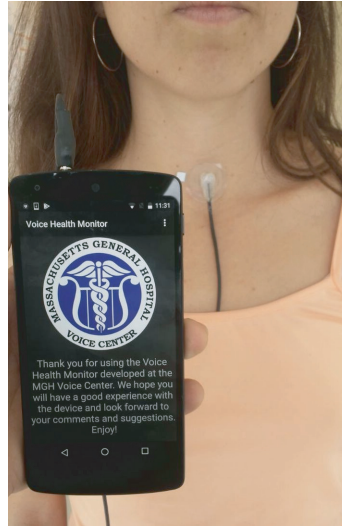
Figure 3.2: Example of VHM system. Illustration of the smartphone-based ambulatory voice monitor that uses a neck-surface accelerometer attached to the skin halfway between the thyroid prominence and the suprasternal notch of a female subject.
