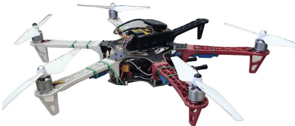
Figure 2.2: A UAV: a common platform to survey large portion of lands and to carry remote sensing devices (Source [1])
