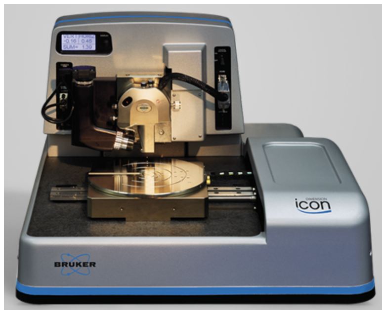
Figure 2.8: C-AFM system (Bruker Dimension Icon) used for topography and current measurements [55].
