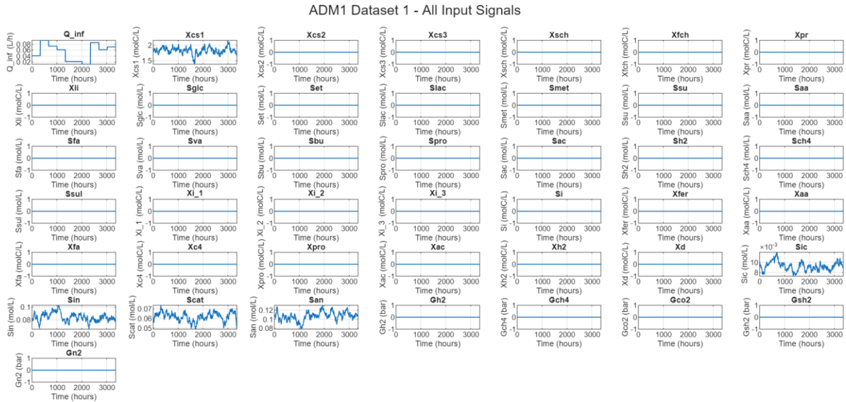
Figure B. 1: Input signals for the ADM1 training dataset, including the manipulated influent flow rate ( Q_{in} ) and stochastic variations in the feed composition.
