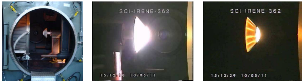
Figure 1.13: IRENE subsystem test in the SCIROCCO plasma wind tunnel at CIRA [75].
