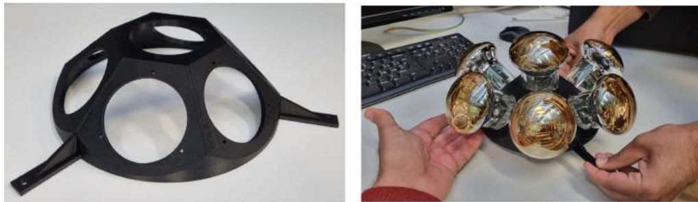
Figure 2.4: Left: 3D printed PMT support structure. Right: The seven PMTs in the support structure. Both from SWGO Collaboration.
