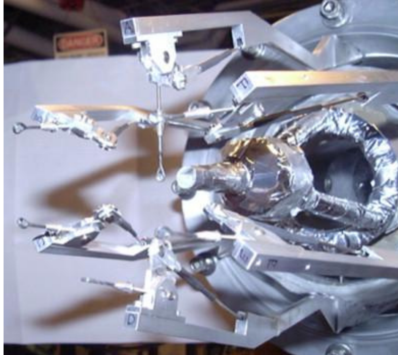
Figure 4.8: Double target support structure with deuterium target's case at the center and one of the solid targets aligned with the beam, attached to the top finger.
