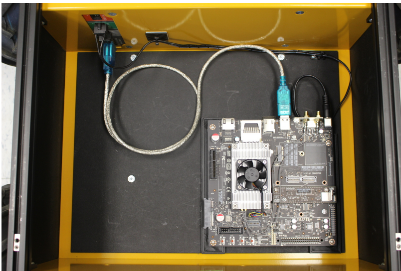
Figure 4.3.: Main computing unit: Nvidia Jetson TX2 developer kit mounted on the Husky A-200 robotic platform.
