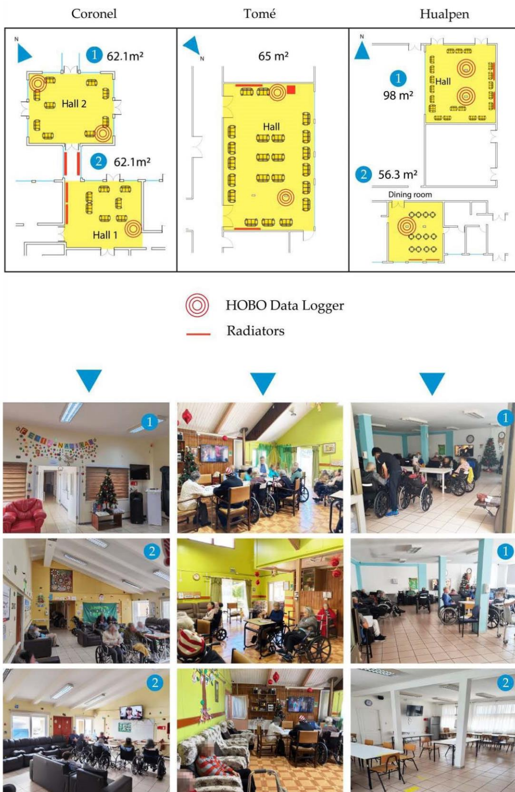
Figure 2. Location of the HOBO dataloggers and representation of the interior spaces subject to temperature monitoring.
