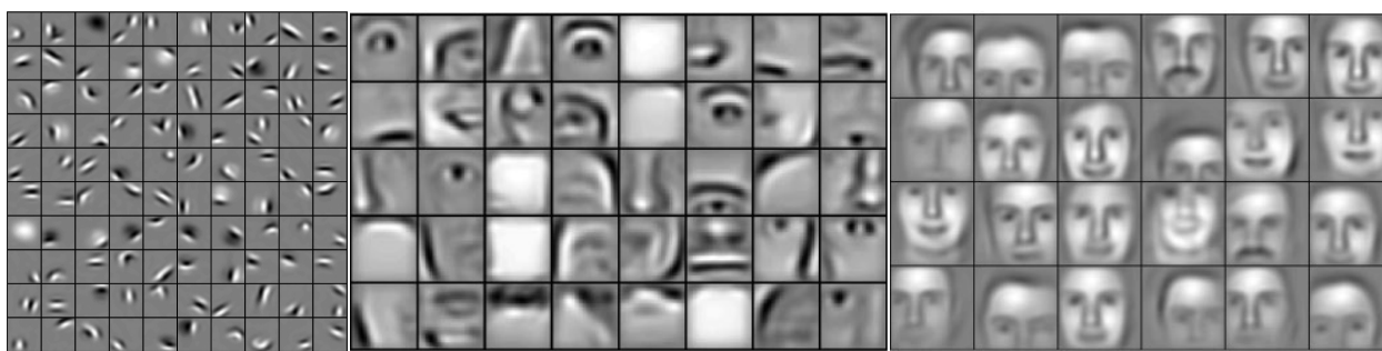
Figure 4.17: Example on the kind of features a CNN could learn in the task of detecting faces. Modified from [71].
