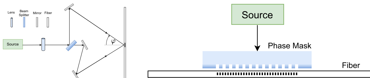
Figure 2.9: Amplitude Splitting interferometer (left). Phase-mask Interferometer (right). The size of the elements are exaggerated for illustration purposes.
