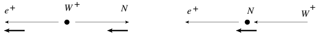
FIG. 3. W^+ \rightarrow e^+N in two frames: the W rest frame (left); the N rest frame (right). Notice that the N spin direction is conserved under the boost.
